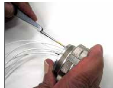
Removal of contacts with metal tool.
