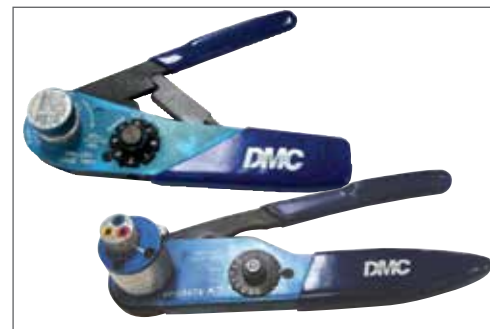
Examples of M22520 Series Crimping Tools: Shown top: tool used for small size 23 contacts.
