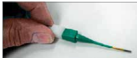
Plastic tool with contact in proper position.
